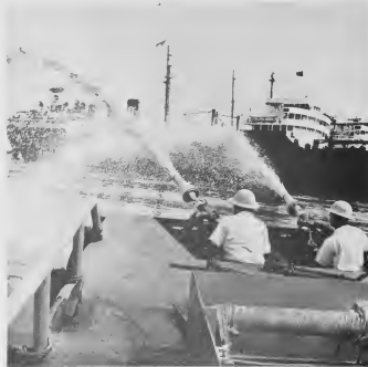
HUNDREDS OF gallons of foam shoot out of the turrets in a scene that resembles combat action aboard a naval vessel. Fire-fighters can handle the turrets with ease and direct foam or water with high accuracy.
